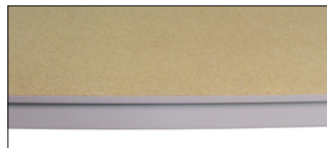
Particle Board Decking
