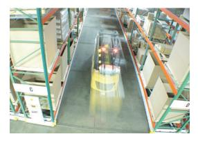
An ActivRAC System can be configured to your application with just one access aisle to accommodate existing fork trucks and pallet racks, to enhance your productivity and reduce driver damage. Remote aisle operation and a fast aisle-opening cycle time helps you maintain or improve your throughput of puts and picks.
