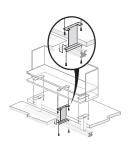
Compose 26"(660mm)H Panel, Connections and Beam — Centered Single Panel Mount — Worksurface to Storage Bracket
